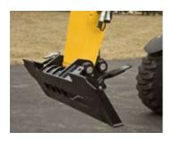
Choose either a telehandler-style coupler, or a universal-style skid steer loader coupler. With either system you can switch Work Tools for added versatility.
